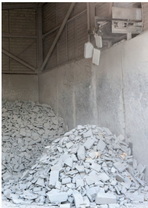
Waste from production of Thermalite aircrete blocks is collected and used to make aggregate blocks.
