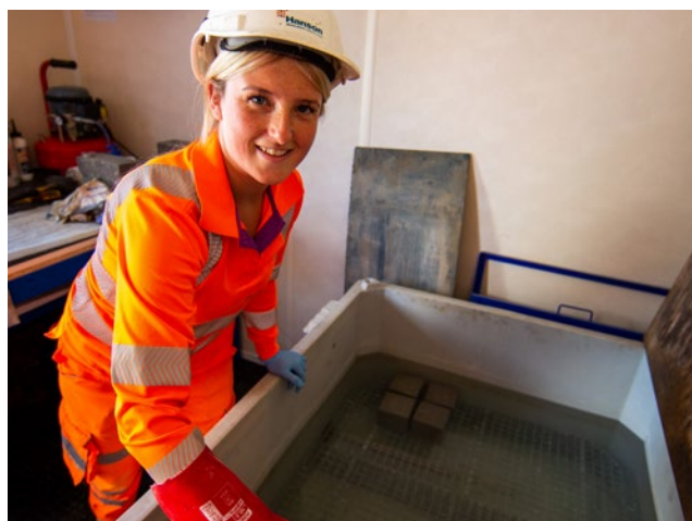
Test concrete cubes at Rochester concrete plant
